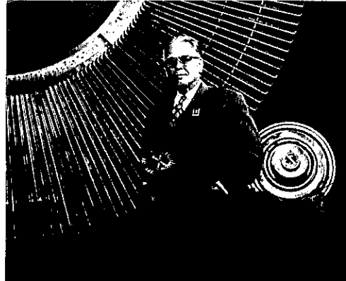
Glenn B. Warren holds smallest GE turbine wheel (6-in. diameter, 34,000 rpm, for supercharger). In background is portion of largest (14 ft. diameter, 1800 rpm, for steam turbine) wheel.
