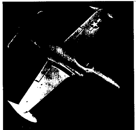
America's first operational jet fighter, the Lockheed P-80 Shooting Star, powered by I-40 (J-33) engine.
