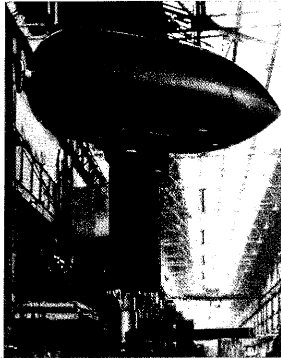
"Zeppelin"-shaped induction motor for Langley Field propeller testing.
