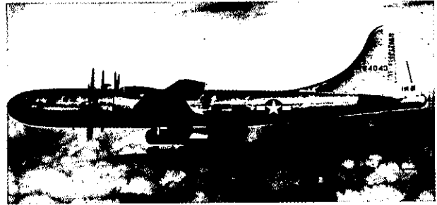
GE's flying laboratory, a U.S. Army Air Force B-29 Superfortress, with jet engine slung under fuselage for testing.
